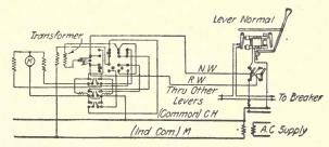
FIG. 148.—Typical control circuit diagram for switch. (Railway Signal Engineer.)
