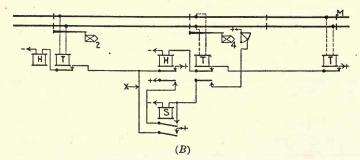
FIG. 281.-A. P. block system circuits.
