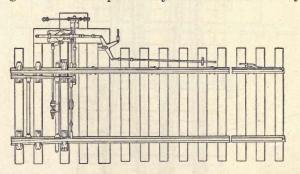
FIG. 73.-Switch and lock movement and bolt lock applied to a switch.
