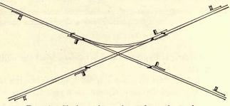
FIG. 25.—Single track crossing and transfer track.
