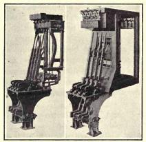
FIG. 143.—"S-7" Electro-mechanical interlocking machine.
