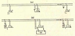
FIG. 154 .- Cut section track circuits.
