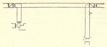
FIG. 243.-Double-rail return. Ironless impedance bonds.
