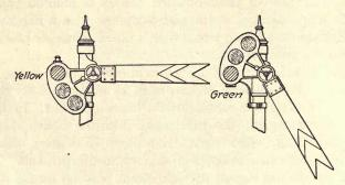
FIG. 3.—Two-position distant signal.
