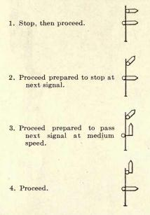
FIG. 220.—Three-block indication scheme.
