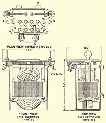
FIG. 246.-Transformer. Closed magnetic circuit type.
