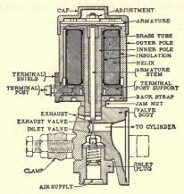
FIG. 104.-Cross-section of pin valve.
