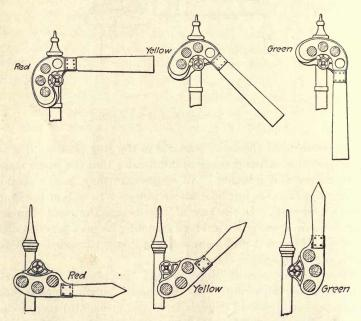
FIG. 4.—Three-position lower and upper quadrant signals.
