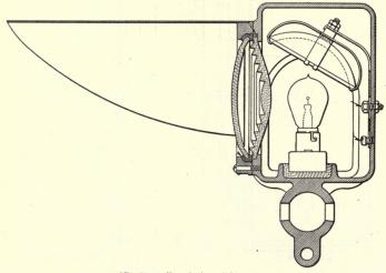
(B) Details of signal lamp.FIG. 317.—Position-light signal. (Union Switch and Signal Co.)
