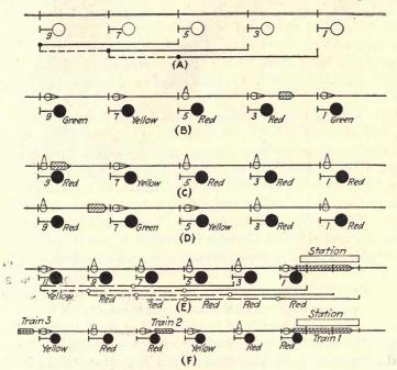
FIG. 265.—Control limits and indications on lines of the New Yo functional Railway Corporation.
