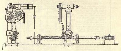
FIG. 85.—One-arm two-position upper quadrant dwarf signal.
