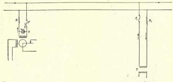
FIG. 238.—Single-rail return. Impedance coil shunting relay.
