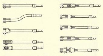
FIG. 51.—Solid and screw jaws.
