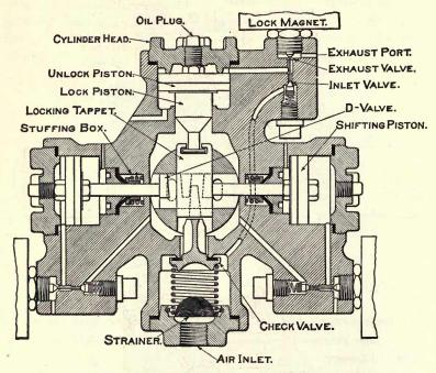
FIG. 103, PART 2 .- Switch valve and magnets.
