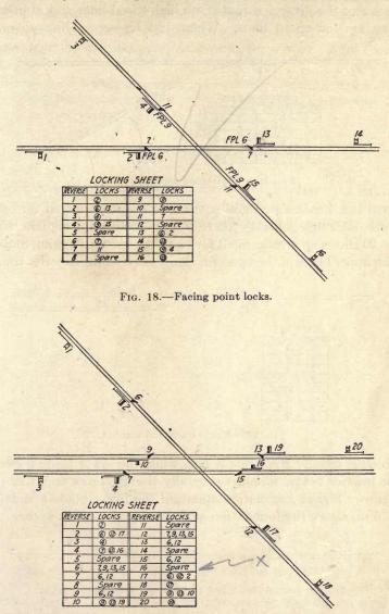
Fig. 19.—Single track crossing a double track.
