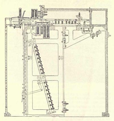
FIG. 151.—Section through Hall interlocking machine.
