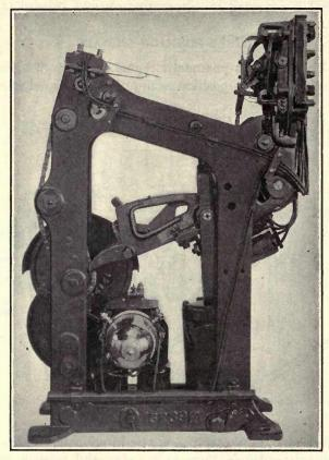
FIG. 295.-Style "S" D.C. motor mechanism.
