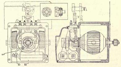
FIG. 308.—Federal type "4" top-post signal mechanism.
