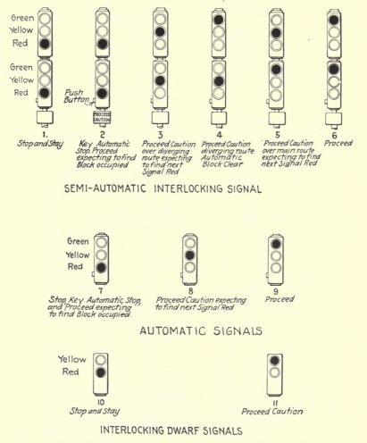
FIG. 314.—Signals used on lines of New York Municipal Railway Corporation. (General Railway Signal Co.)
