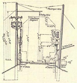
FIG. 286.—Arrangement of apparatus at double signal location, C. M. & St. P. Ry. (Proceedings, R. S. A., 1917.)
