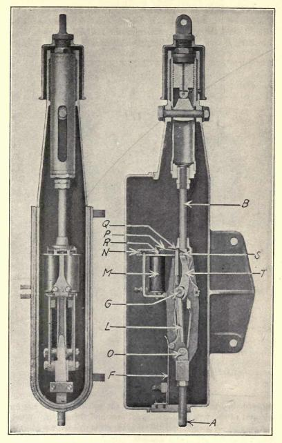
FIG. 195.—Union electro-mechanical slot.
