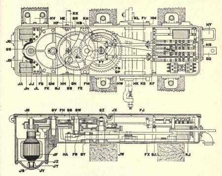
FIG. 147.-Type 41 switch machine.
