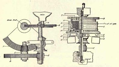
FIG. 304.—Operating mechanism for style "K" signal.
