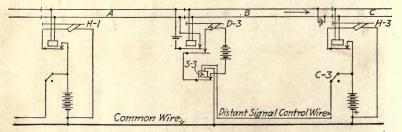
FIG. 222.-Wiring diagram for one-arm two-position signals.
