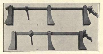
FIG. 46.-Rocking shafts for leadouts.
