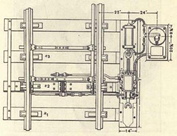
FIG. 101.-Electro-pneumatic switch and lock movement.
