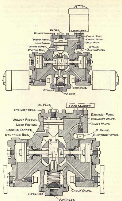
FIG. 103, PART 1 .- Switch valve and magnets.
