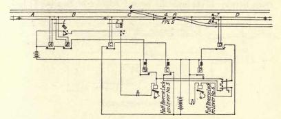
FIG. 191.—Approach and route locking. R. S. A. plan 1149.
