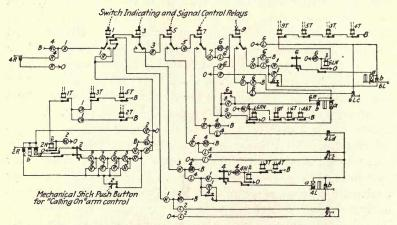
FIG. 142.-Signal control circuits for Fig. 141.
