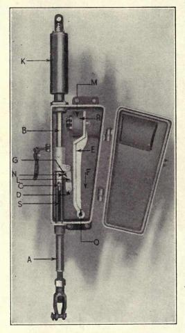
FIG. 196.—Hall electro-mechanical slot.
