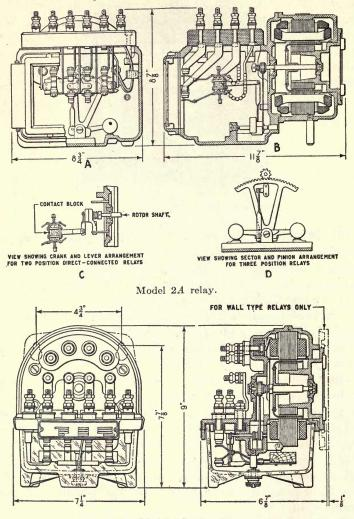
Model 2B relay. Fig. 254, part 1. Models 2A and 2B relays.
