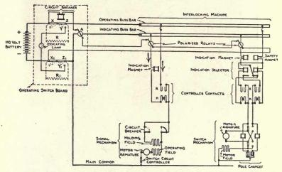
Fig. 133.—Circuits for operating switchboard, interlocking machine and switch and signal functions.
