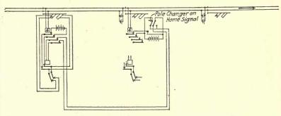
FIG. 228.—R. S. A. diagram for two-arm two-position signals. Polarized line circuits. (Plan 1078A, page 369, Proceedings 1910.)
