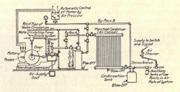
FIG. 92.—Diagram of typical air compressing, cooling and distributing system for electro-pneumatic interlocking.
