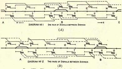
FIG. 277.—Three-position signals for single-track.
