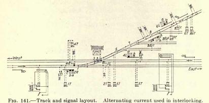
signal is cleared, a check is provided that the switches are properly set, that the switches correspond with their levers, and that no switch is manually operated or even unlocked after the indication is received. The route to be properly set for one signal must be
