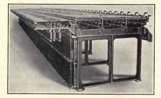
FIG. 95.-Electro-pneumatic interlocking machine. Rear view.
