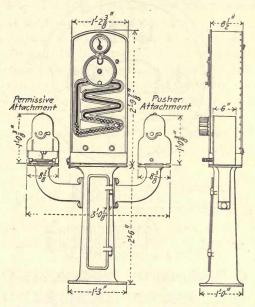
FIG. 210.—Permissive and pusher attachments.
