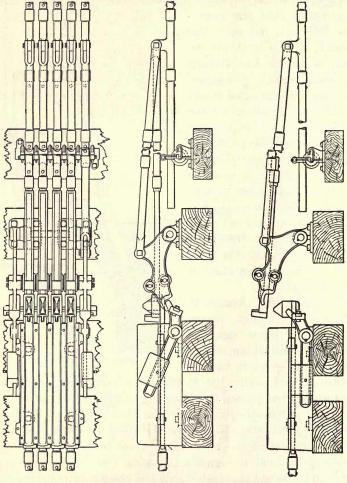
FIG. 89.-Swing bridge coupler. (Signal Dictionary.)
