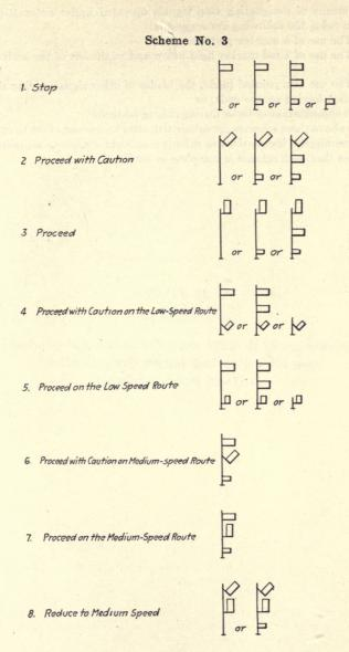
As means of designating stop signals operated under automatic block system rules, the following are suggested:
