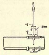
FIG. 68.—One-way bolt lock.
