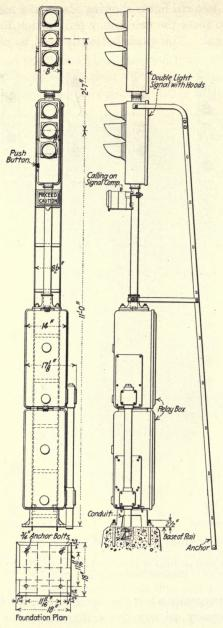
FIG. 315.—Interlocking signal shown in Fig. 314.
