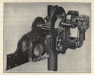
FIG. 296.—Style "T-2" D.C. signal mechanism. Parts cut away to show construction.
