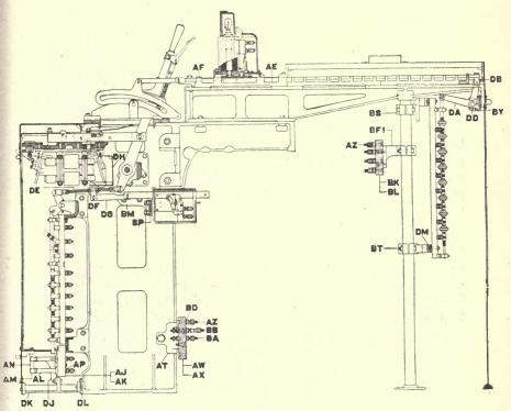
FIG. 146.-Section through Federal interlocking machine.
