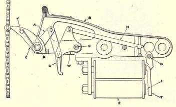
FIG. 292.-Style "B" slot arm.
