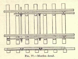
for clearing or derailing trains. This type is used principally on high-speed routes.
