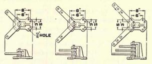
FIG. 60.-R. S. A. one-, two-, and three-way cranks.
