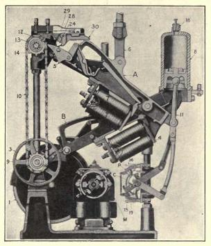
FIG. 290.-Style "B" two-position signal mechanism.
