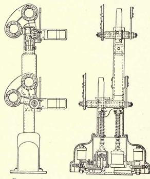
FIG. 111.-Two-arm electro-pneumatic dwarf signal.
