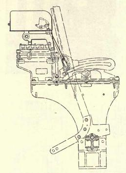
FIG. 179.-Electric lock applied to a mechanical interlocking machine.
