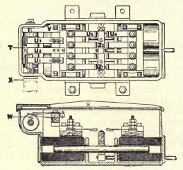
FIG. 123.—Pole changer for Model 2 switch machine.
