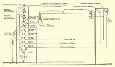
FIG. 110.—Diagram of complete control, indication and locking circuits for single switch with D.C. indication.
