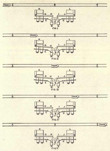
FIG. 326.-Diagram showing operation of Union interlocking relay.
