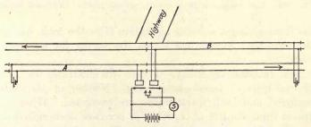
FIG. 324.-Low voltage signal circuit for double-track line.
