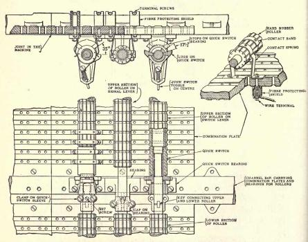
FIG. 100.-Rollers, contact springs and quick switches.
