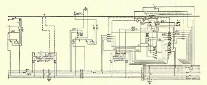
FIG. 283.-A. P. block system on the Puget Sound Electric Railway.
