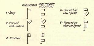
As means of designating stop signals operated under automatic block system rules, the following are suggested:
