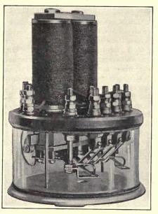
FIG. 160.-Neutral relay. (Union Switch & Signal Co.)
