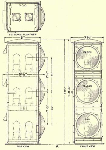
FIG. 316.—Subway and tunnel signal. (Union Switch and Signal Co.)
