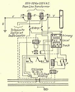
FIG. 263.-Typical circuits used on the Southern Railway.
