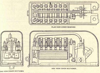
FIG. 180.-Details of electric lock.
