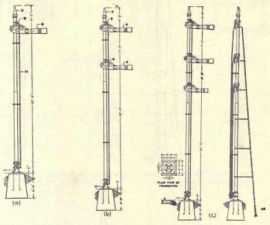
FIG. 81.-R. S. A. standard upper quadrant signals.
