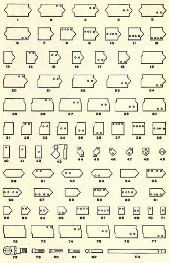
FIG. 40.-Locking details of style A interlocking machine.
