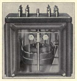
FIG. 251.-Centrifugal frequency relay.
