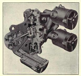
FIG. 102.—Switch valve and magnets.
