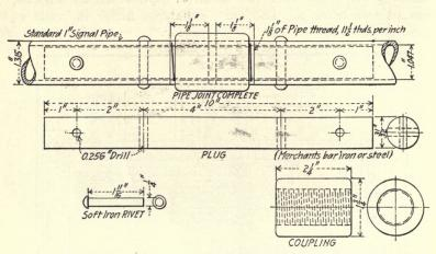
FIG. 50.-R. S. A. 1-in. pipe and coupling.
