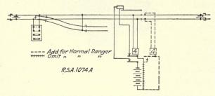
FIG. 235.—R. S. A. normal clear circuits for trailing switch and curve protection. Traffic in one direction. (*Plan 1074A*, page 365, *Proceedings* 1910.)
