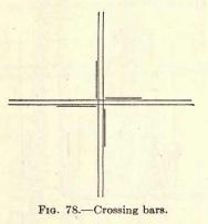
car or locomotive is standing on a railroad crossing. They are just ordinary detector bars placed as near to the crossing frog as possible, one on each side of the crossing in each track. These bars lock the derails both normal and reversed so that they cannot
