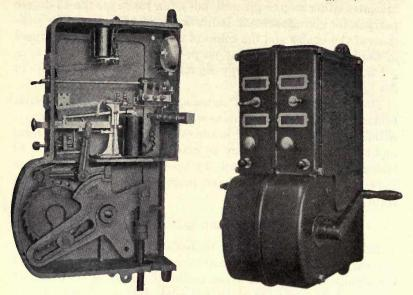
FIG. 200.-Controlled-manual station block instrument.
