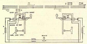
FIG. 194.—Check locking circuit. direction of traffic. (General Railway Signal Co.)
