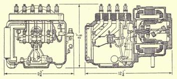
FIG. 255.—A. C. relay. Model 2A, two-position centrifugal frequency type. Rotor operated.
