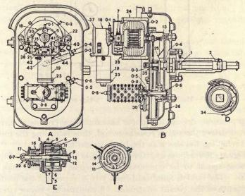
FIG. 297.-Diagram of style "T-2" D.C. signal mechanism and parts.
