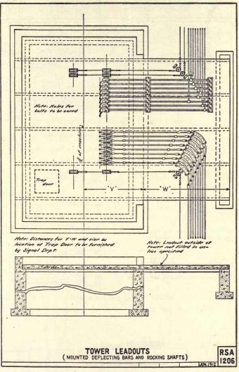
FIG. 49.-R. S. A. tower leadout.
