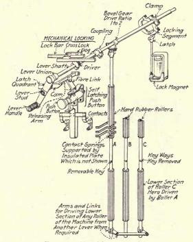
FIG. 98.—Signal lever complete.
