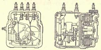
Model 2B, time element relay. Fig. 254, part 2. Models 2A and 2B relays.
