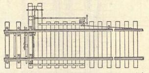
FIG. 72.-Facing point lock and bolt lock applied to a switch.
