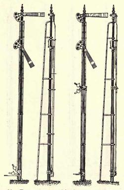
FIG. 80.—Two-arm two-position lower quadrant signals.
