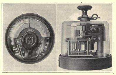
FIG. 187.-Clock-work time release.
