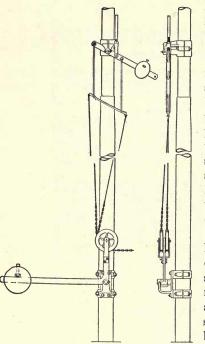
FIG. 59.-Wire compensator.
