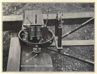
FIG. 329.-Style "A" generator with cover removed.
