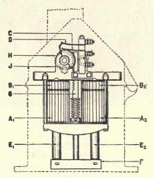
FIG. 130.-Model 2 solenoid dwarf signal operating mechanism.
