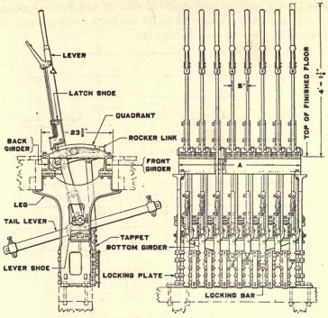
FIG. 37.-Style A interlocking machine.
