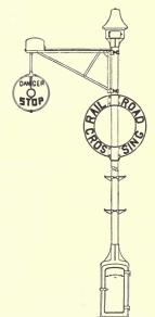
FIG. 321.—Wigwag crossing signal. (Railroad Supply Co.)
