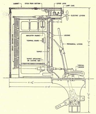
FIG. 135.—Electro-mechanical interlocking machine.
