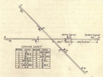
FIG. 16.—Single track crossing a single track.
