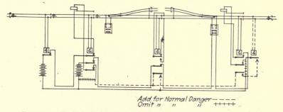
FIG. 234.—R. S. A. design for protecting obscure curves and switches. (*Plan 1075A*, page 366, *Proceedings 1910.*)
