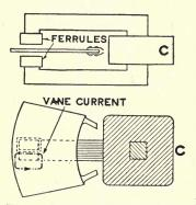
Fig. 247.—Operating element of vane relay.
