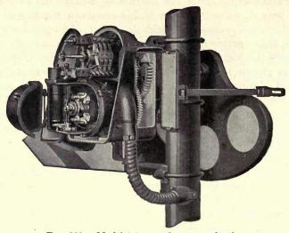
FIG. 299.-Model 2A, top-of-mast mechanism.
