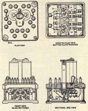
FIG. 161.-Polarized relay.
