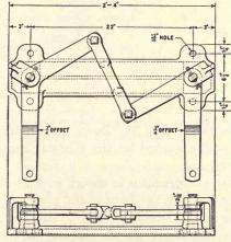
FIG. 55.-R. S. A. "lazy jack" pipe compensator.
