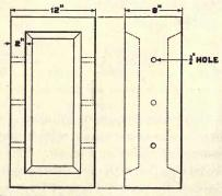
FIG. 64b.-R. S. A. pipe carrier foundation.
