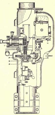
FIG. 305.—Operating mechanism for style "K" signal.
