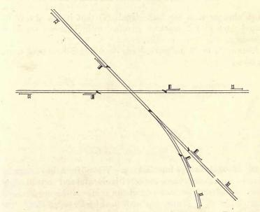
FIG. 24.-Single track crossing and high speed diverging route.
