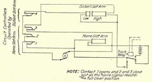
FIG. 291.—Wiring diagram for style "B" signal when operated by direct current and controlled by polarized relay.
