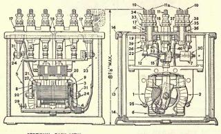
SECTIONAL BACK VIEW SECTIONAL SIDE VIEW FIG. 250.—Iron core galvanometer relay.
