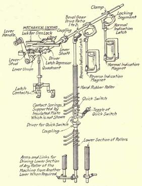
FIG. 96.—Switch lever complete.
