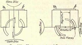
FIG. 289.-Electro-magnets and Z-armature.
