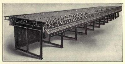
FIG. 94.-Electro-pneumatic interlocking machine. Case removed.
