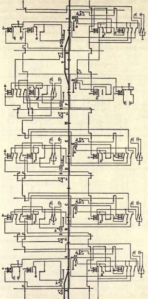
FIG. 282.-A. P. block system circuits.
