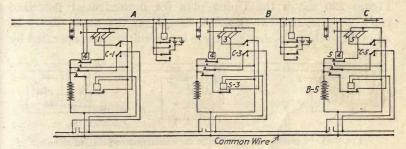
FIG. 223.- Two-arm two-position signal circuits.
