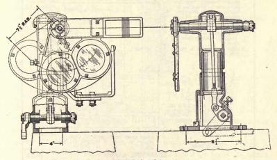
FIG. 86.-R. S. A. dwarf signal for pipe connection.
