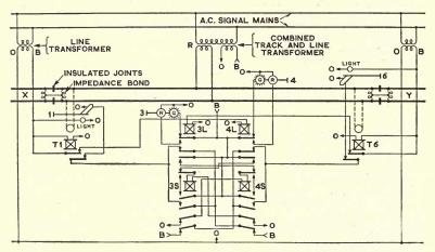
FIG. 275.—Circuit scheme for TDB system.
