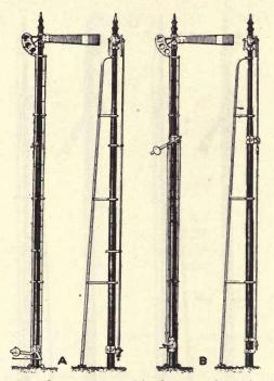
FIG. 79.-One-arm two-position lower quadrant signals.
