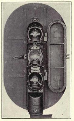
FIG. 313.—Union Model "N" light signal. Rear view.
