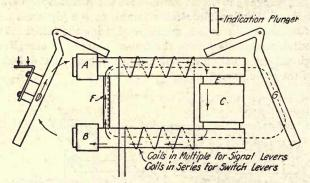
FIG. 149.—The safety and indication magnet. (Railway Signal Engineer.)
